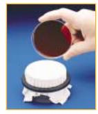
colonies in the new dish. The replica-plating device may be disinfected between uses with a brief rinse in ethanol or chlorine bleach. The aluminum ring is 102mm diameter and the PVC cylinder is 55mm high. For use with 90 to 100mm petri dishes. One bag of 12 Velveteen Squares is included.
